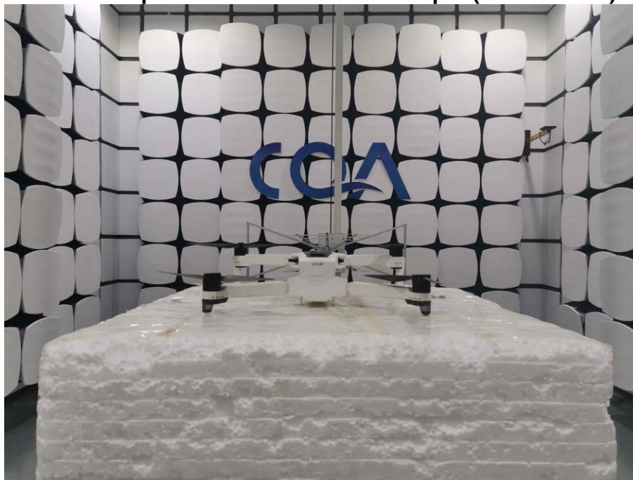
Radiated spurious emission Test Setup-1 (Below 1GHz)
