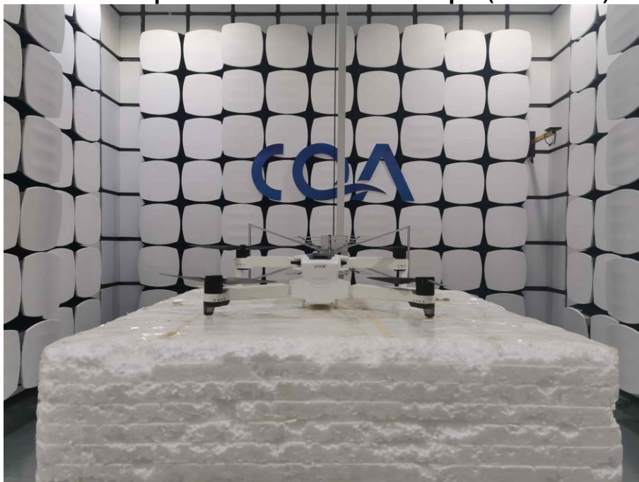
Radiated spurious emission Test Setup-1 (Below 1GHz)
