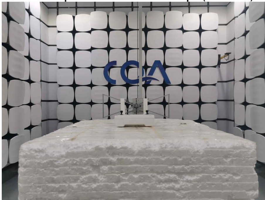
Radiated spurious emission Test Setup-1 (Below 1GHz)
