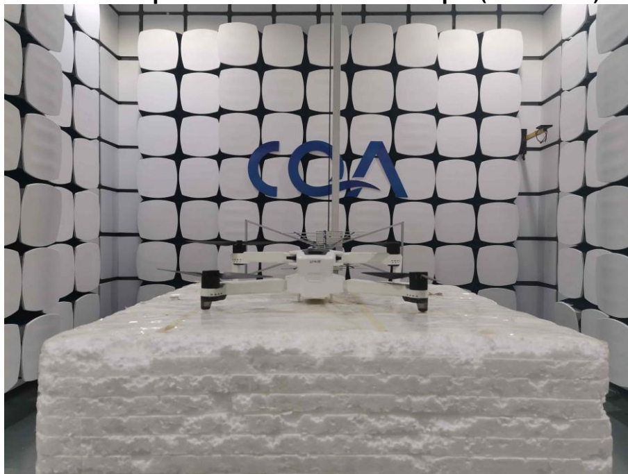
Radiated spurious emission Test Setup-1 (Below 1GHz)
