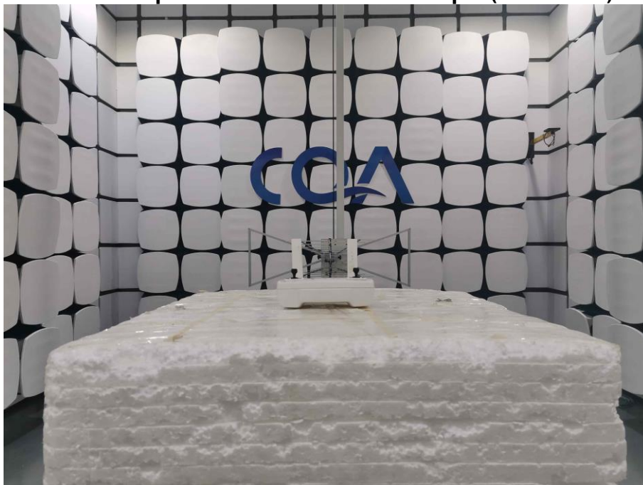
Radiated spurious emission Test Setup-1 (Below 1GHz)
